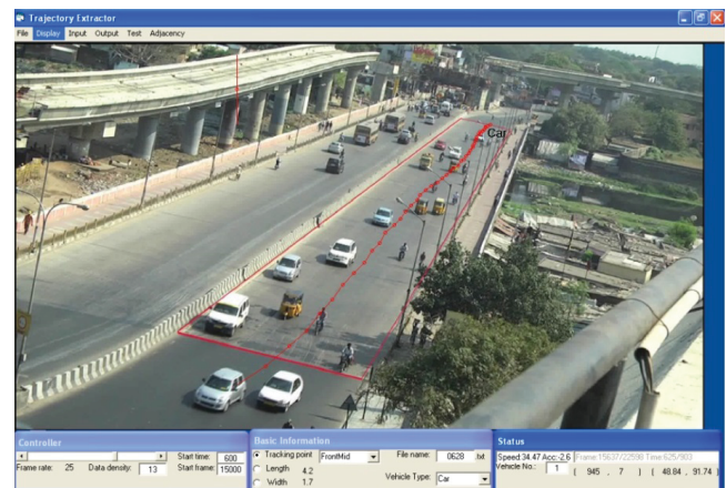
FIGURE 2 Trajectory extractor user interface showing road section and reference points.
