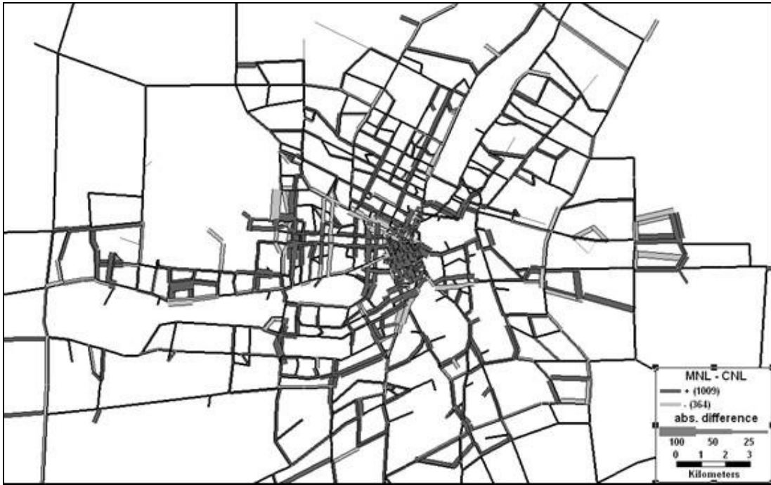
Figure 7 Difference in link flows between MNL-SUE and CNL-SUE models.
