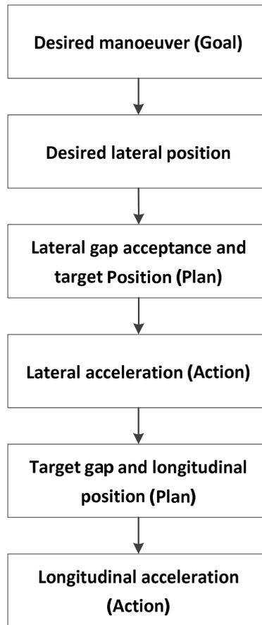
**Figure 11 Overall Model Framework for Driver Behavior in Mixed Traffic**
