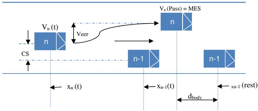
**Figure 6 Speed to Allow Partial Lane Change (adapted from [30])**
