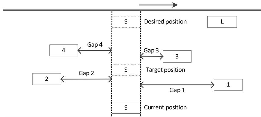
**Figure 13 Lateral Gap Acceptance and Target Position**
