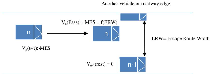
**Figure 5 Speed to Allow Squeeze Pass the Leader (adapted from [30])**
