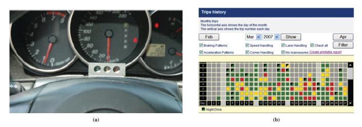
FIGURE 1 Feedback media: (a) in-vehicle display and (b) web-based application.
