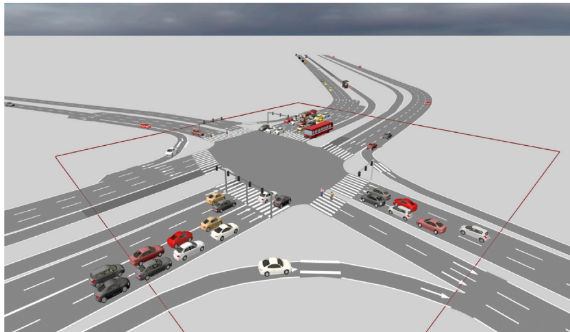
Fig. 14. Case study intersection modeling by the microscopic simulation model Aimsun.
